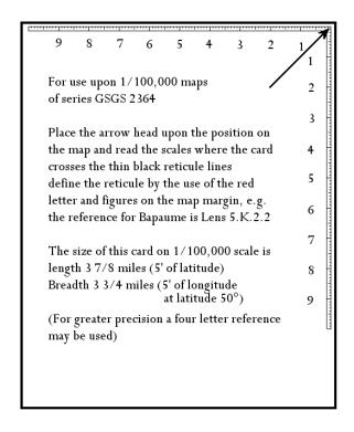
squares or rectangles or sectors, which can be defined by reference numbers or letters. To facilitate the use of coordinates on the maps, special cards have been prepared and issued. Diagram 2 shows the cards for the 1:20,000 and 1:10,000, and for the 1:100,000 scales. The two large scales are at opposite ends of the same card.
