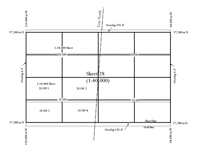
NOTE.—Amount of overlap and inclination of meridian have been exaggerated for clearness.
